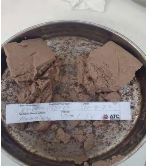
Sample after shearing, sliced down center.
