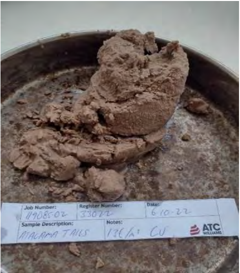
Sample after removal from membrane.
