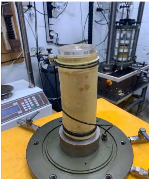
Sample prior to shearing.
