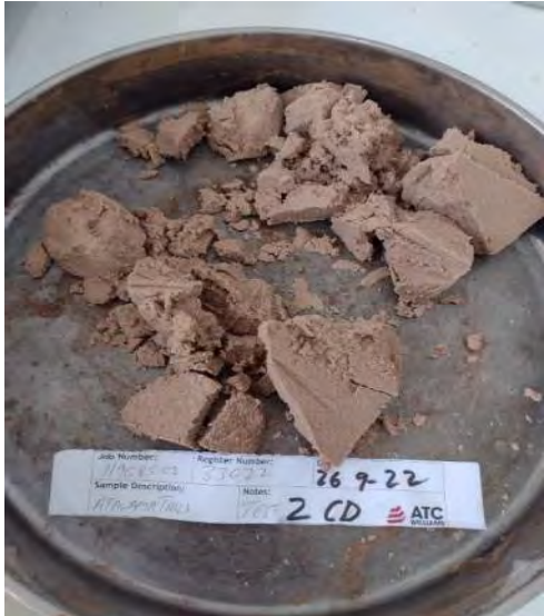
Sample after shearing, sliced down center.
