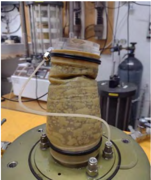
Sample after shearing, still within membrane.
