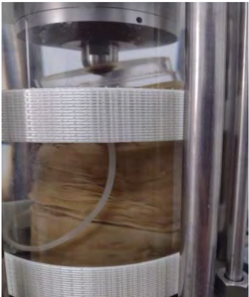
Sample after shearing, still within membrane.
