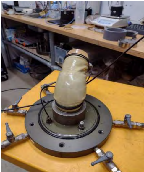
Sample after shearing, still within membrane.
