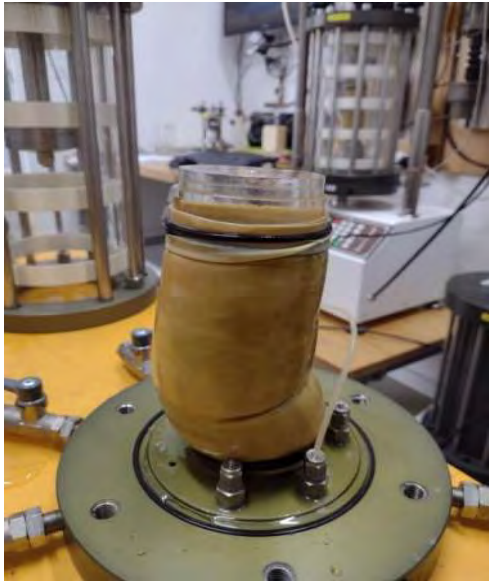
Sample after shearing, still within membrane.
