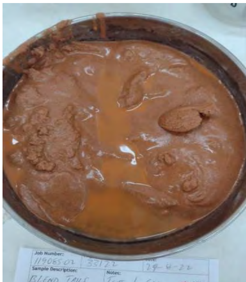
Sample after shearing, sliced down center.
