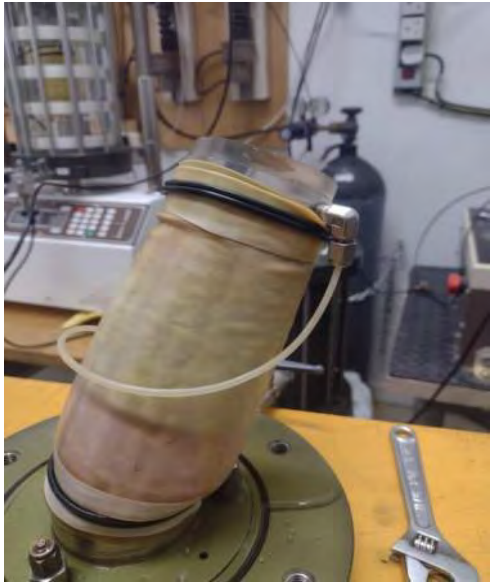
Sample after shearing, still within membrane.
