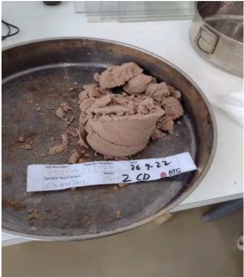
Sample after removal from membrane.
