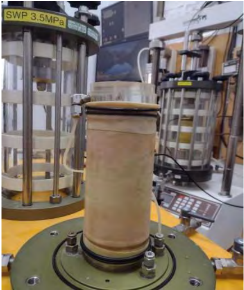
Sample prior to shearing.
