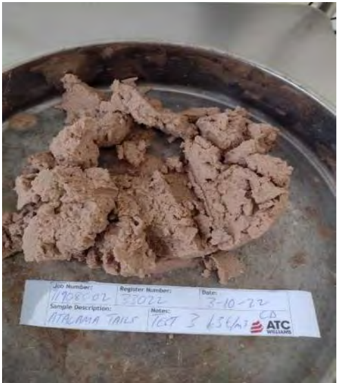
Sample after shearing, sliced down center.
