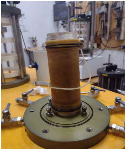
Sample prior to shearing.
