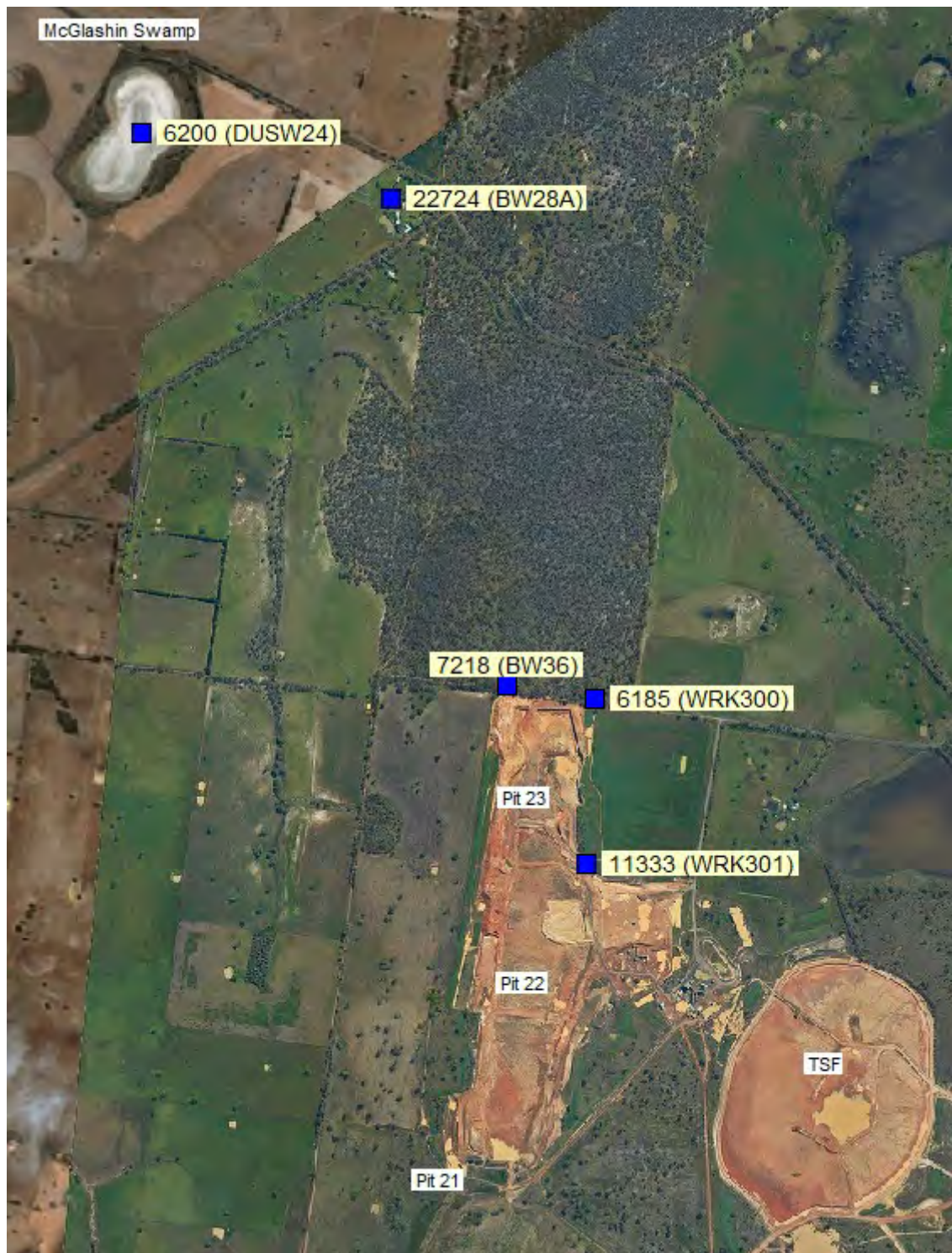
Figure 3.5 Locations and latest (2018) electrical conductivity measurements ( \mu\text{S}/\text{cm} ) of bores in or near the groundwater flow path from Pit 23 and at McGlashin Swamp (DUSW24)
