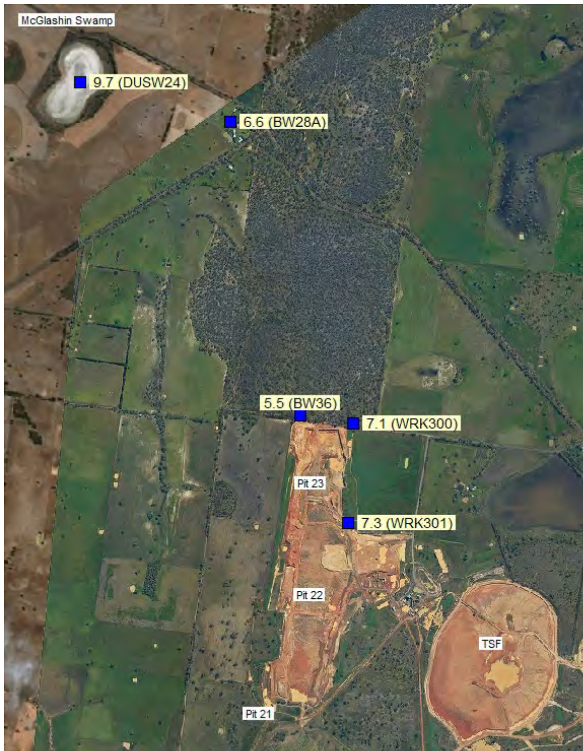
Figure 3.10 Locations and latest (2018) pH measurements of bores in or near the groundwater flow path from Pit 23 and at McGlashin Swamp (DUSW24)
