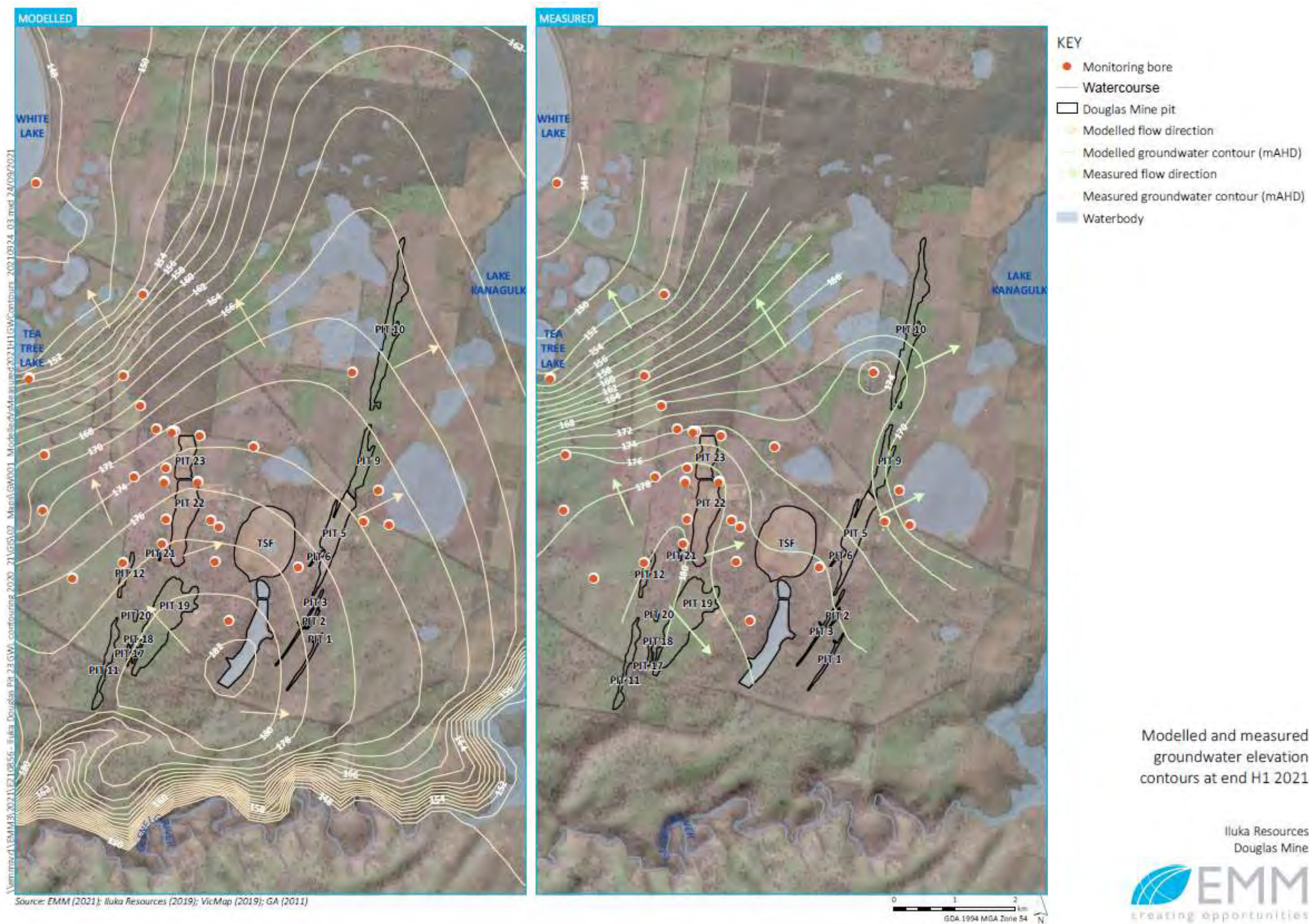
Figure 17: 2019 modelled vs 2021 interpreted groundwater contours (EMM 2019; EMM 2021)
