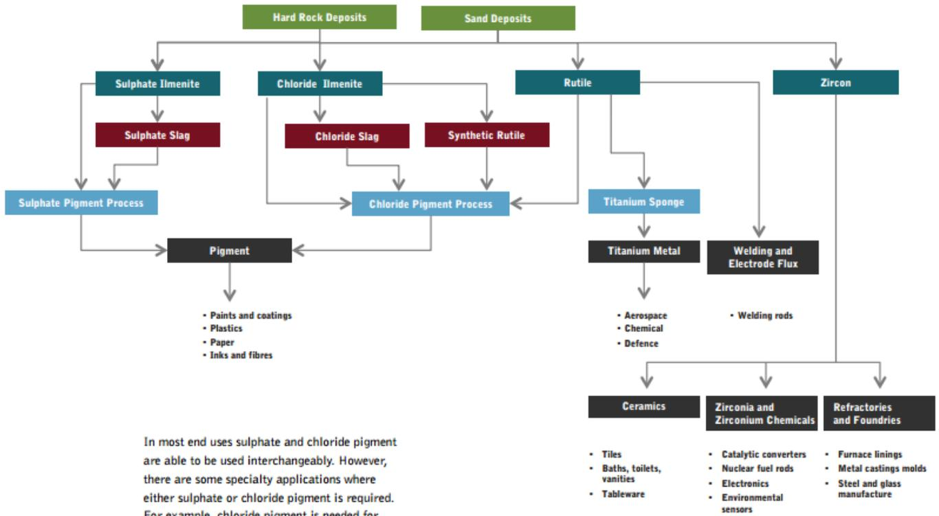
The mineral sands industry involves the mining and processing of zircon and titanium dioxide products (ilmenite, rutile and upgraded titanium dioxide products of synthetic rutile, slag and upgraded slag). The two product categories have different properties, prices and distinct end use markets.
