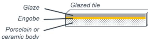
Zircon contained mainly in engobe (~6-12% zircon) and glaze (~8-16% zircon).
